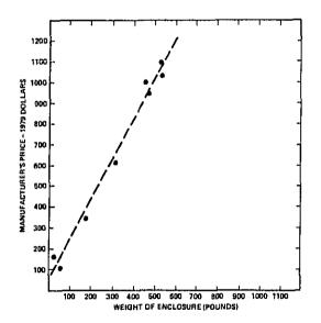
FIG. 25. RELATIONSHIP BETWEEN ENCLOSURE WEIGHT AND MANUFACTURER'S PRICE.
