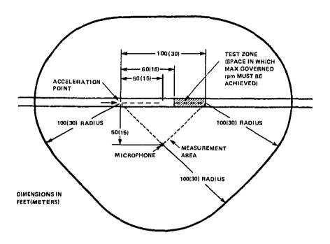
FIG. A.1. TEST SITE FOR EXTERIOR NOISE LEVEL MEASUREMENTS.
