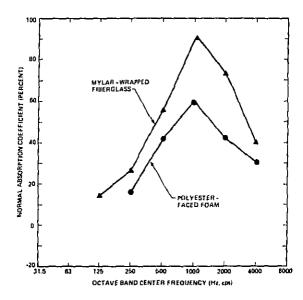
FIG. 13. NORMAL SOUND-ABSORPTION COEFFICIENTS FOR POLYESTER-FACED FOAM AND MYLAR-WRAPPED FIBERGLASS.
