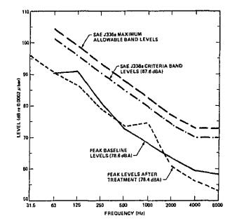
FIG. 22. INTERIOR NOISE LEVELS COMPARED WITH SAE J336a CRITERIA.
